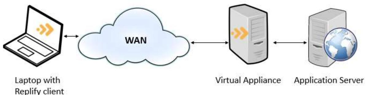
In this deployment, clients are installed on individual end user machines and these are configured to connect to either a Virtual Appliance or to a REM. This can be useful when clients are on mobile devices such as laptops or where the infrastructure isn't available to install a peered appliance.
