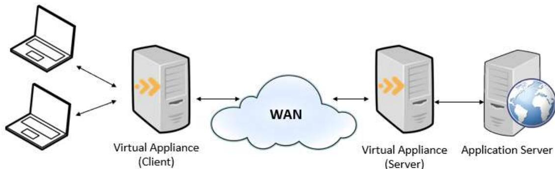
The peered appliance deployment model can be used when there are several devices requiring optimization at a single location. In this model a Virtual Appliance is deployed at both ends of the network link. Traffic from the site that is remote to the Application Servers needs to be routed via the local Virtual Appliance using one of the following mechanisms.
